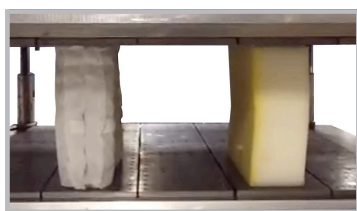
Deflection test – Quantum Edge vs. standard foam encasement
