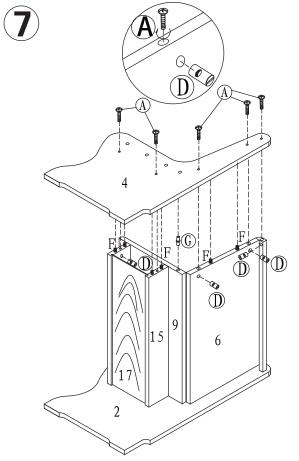
Assemble Short Nook Side(4) to Assembled Unit with Bolt(A), Screw Nut(D) and Glue(F) as shown.
