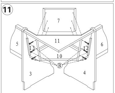
Assemble Conner Back Rest(7) to Wings(12&13) with Screw(B) as shown
