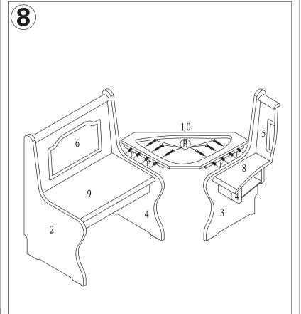
Assemble Conner Seat(10) to assembled unit with Screw(B) and Glue(F) as shown.
