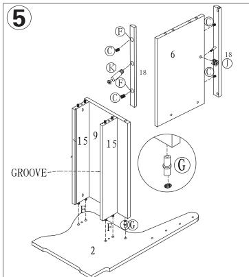
Attach Wooden Dowel(C) and Assemble Camlock Bolt(K) to Short Seat Back Bar(19)With Glue(F), Then Assemble to Short Seat Back(5) with Glue(F) and Camlock(J) As Shown. Attach Short Storage Shelf Rails(15) to Short Nook Side(2) with Glue(F), and Attach Short Seat Bench(9) to Short Nook Side(2) With Pivot Pin(G).
