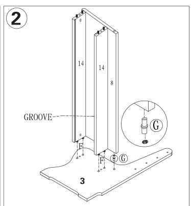
Attach Long Storage Shelf Rails(14) to Long Nook Side(3) with Glue(F), and attach Long Seat Bench(8) to Long Nook Side(3) with Pivot Pin(G).
