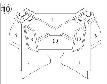
Assemble Conner Top Shelf(11)to Wings(12&13) with Screw(B) As shown.
