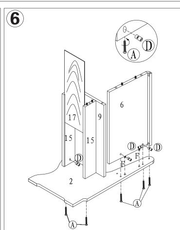
Assemble Short Storage Shelf Rails(15) and Short Seat Back(6) to Short Nook Side(2) with Bolt(A), Screw Nut(D) and Glue(F) as shown. Then insert Short Shelf Base(17) to Assembled Unit.
