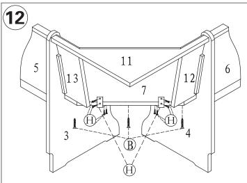
Assemble Conner Seat(10) to Conner Back Rest(7) with two Conner Brackets (I) by using Screw(H) and screw(B) as shown.
