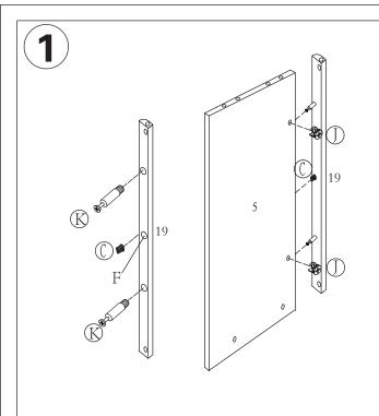
Attach Wooden Dowel(C) and Assemble Camlock Bolt(K) to Long Seat Back Bar(19)With Glue(F), Then Assemble to Long Seat Back(5) with Glue(F) and Camlock(J) As Shown.
