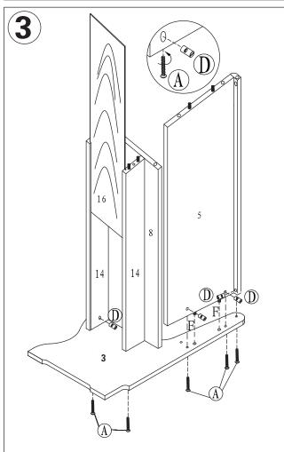
Assemble Long Storage Shelf Rails(14) and Long Seat Back(5) to Long Nook Side(3) with Bolt(A) ,Screw Nut(D) and Glue(F) as shown. Insert Long Shelf Base (16) to Assembled Unit as shown.
