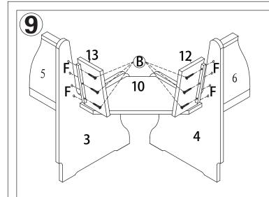
Assemble the two Wings(12&13) to Assembled Unit with Screw(B) and Glue(F) as shown.
